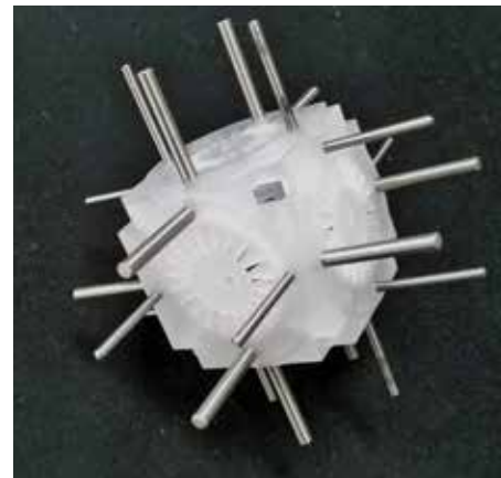
Precision metal press fit dowel pins on all orthogonal sides of a cube
