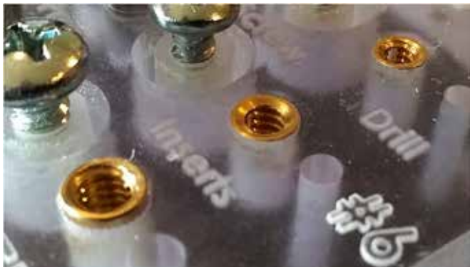
Fourth column from left shows brass screw-to-expand inserts. These can be inserted with either an arbor press or a hammer
