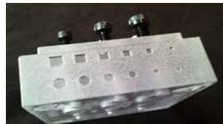
Square and round features on the sides of the diagnostic show isotropic properties
